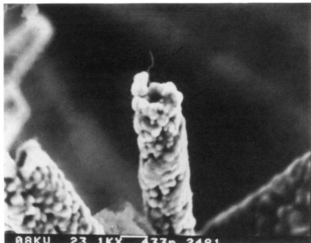
Figure 4. SEM of nickel-silica coated tubules. The sample was air-dried on the SEM stage from an acetone dispersion.
